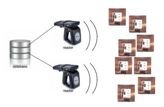
Figure 1. RFID architecture
