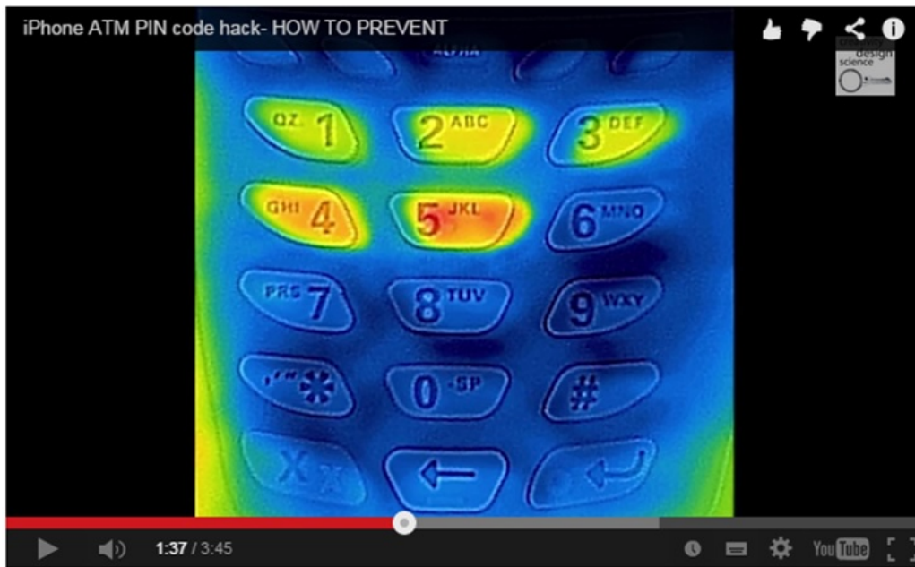
Figure 9.3: Still from video claiming PINs can be captured with FLIR ONE
