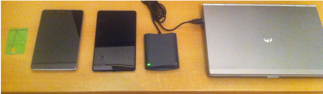
Figure 6.2: Our test relay setup: (from left to right) bank card, Mole Device, Relay Device, emulated POS terminal)
