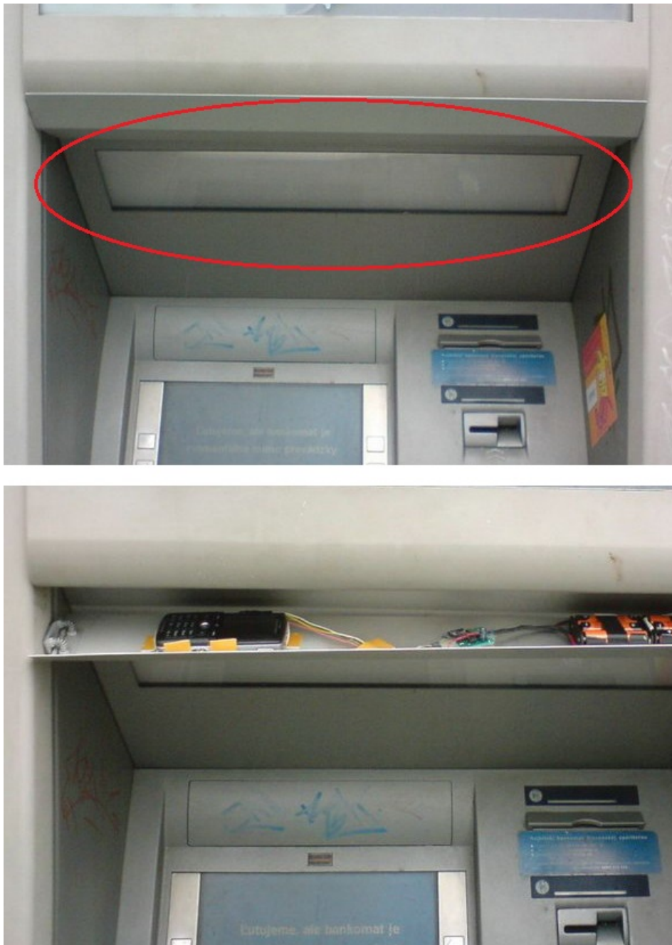
Figure 9.1: An improvised camera solution used for recording PINs (Source 47 )
