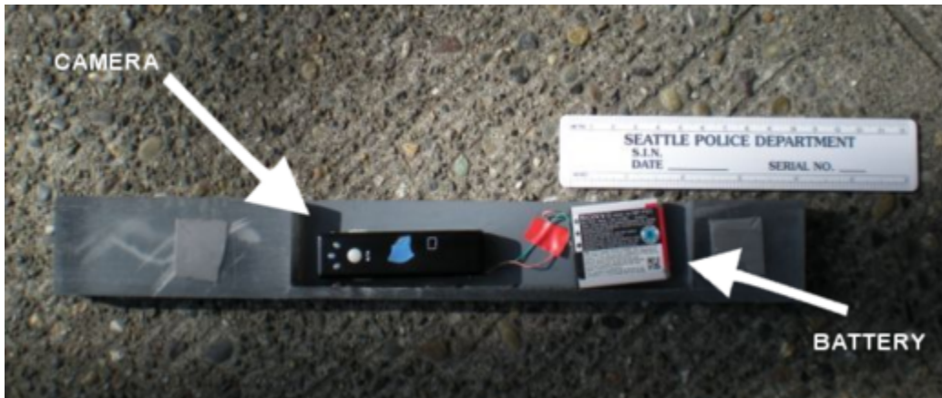
Figure 9.2: A very small camera used for recording PINs (Source 48 )
